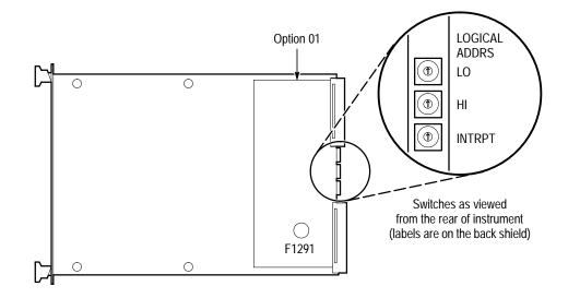
Figure 1–1: Option 01 Indicators and Switch Locations
